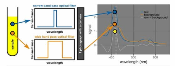
FIGURE 18: Proposed method of using photography to acquire background-subtracted signals with a narrow band pass optical filter and a wide band optical filter.
