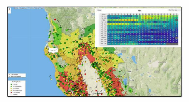
FIGURE PG&E-7.3.2-8: THE PWAS THAT DISPLAYS AND ALSO DISSEMINATES ALERTS WHEN WIND SPEEDS EXCEED THRESHOLDS – USERS CAN CUSTOMIZE ALERTS TO ONLY RECEIVE ALERTS FOR THE AREA(S) NEEDED
