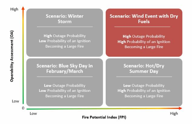
PG&E partnered with a third party to develop the OA Model for transmission. This model combines historical wind speeds for each structure, historical outage activity, and the condition of assets based on inspection programs to help understand the wind-related failure probability of each structure. The OA Model can be driven with forecast wind speeds to output the probability of failure at the structure level each hour.
