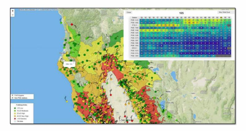
FIGURE PG&E-7.3.2-8: THE PWAS THAT DISPLAYS AND ALSO DISSEMINATES ALERTS WHEN WIND SPEEDS EXCEED THRESHOLDS – USERS CAN CUSTOMIZE ALERTS TO ONLY RECEIVE ALERTS FOR THE AREA(S) NEEDED
