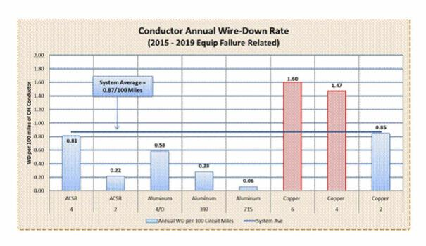
FIGURE PG&E-4.6-1: CONDUCTOR ANNUAL WIRE-DOWN RATE
